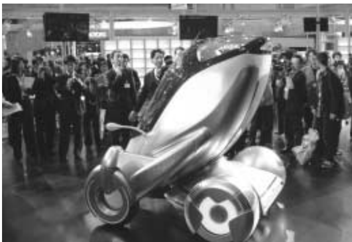
Toyota PM - 'Personal Mobility' one seat concept vehicle using advanced telematics and drive-by-wire technology
