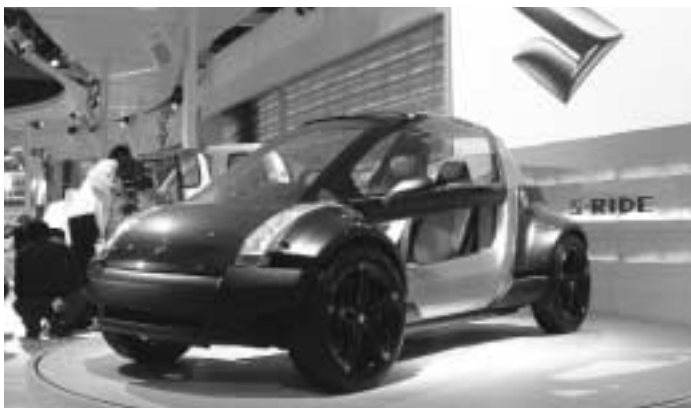
Suzuki S-Ride - an active commuter concept vehicle with motorcycle-like driving (2 seats in tandem)
